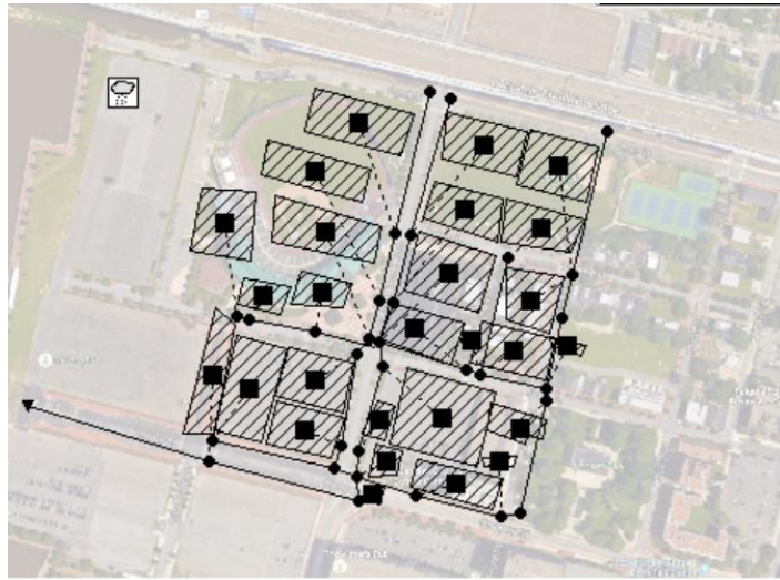
Figure 14. A Portion of Stormwater Sewer System in Camden, New Jersey Modeled in SWMM.
